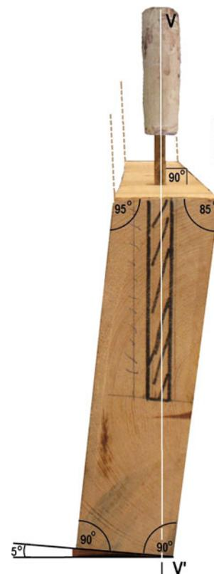
**Fig. 3** Mortise cut at an angle for securing the proper plank inclination after tenon insertion
